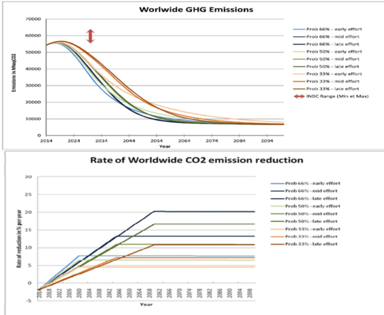
Figure 3 - GHG emission trajectories (MtCO<sub>2</sub>e) without negative emissions for different probabilities of reaching the 2°C target and different maximum effort dates; compared with global 2030 emissions from the aggregation of INDCs and “current policies” scenario (top). Associated emissions reduction rate (bottom).
